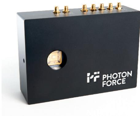
The PF32 comprises a single-photon sensitive imaging sensor with best-in-class timing resolution and a market-leading throughput of up to half a billion photons time-stamped per second.
